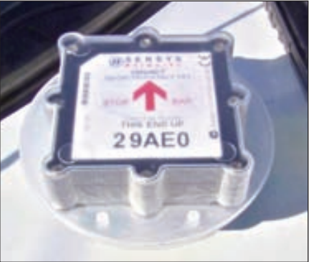
KENTUCKY TRANSPORTATION CABINET Above, workers with a Kentucky Transportation road crew install a new "puck" traffic-detection device at an intersection in Hopkinsville. At right, the device, which is buried in the pavement and covered with epoxy, is shown.
